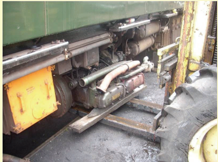
Sc51367's No2 engine during removal, 17/8/12 (B.Faulkner)
