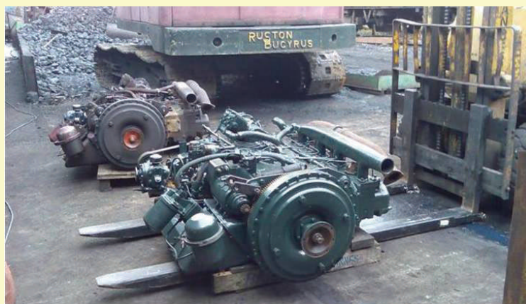
New Engine ready for installation under 50528 (Llangollen Railcar Group)
